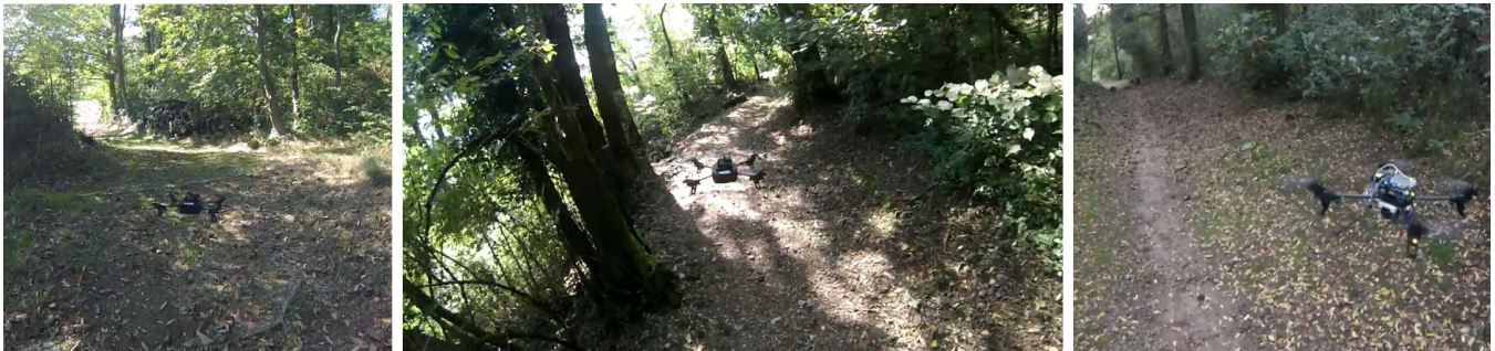
Fig. 6: Images from preliminary field testing. Rightmost figure shows quadrotor with Odroid-U3 featuring full on-board processing.
