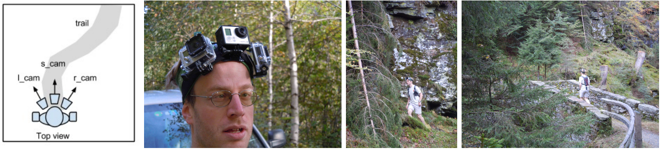
Fig. 2: Left : stylized top view of the acquisition setup; Right : our hiker during an acquisition, equipped with the three head-mounted cameras.
