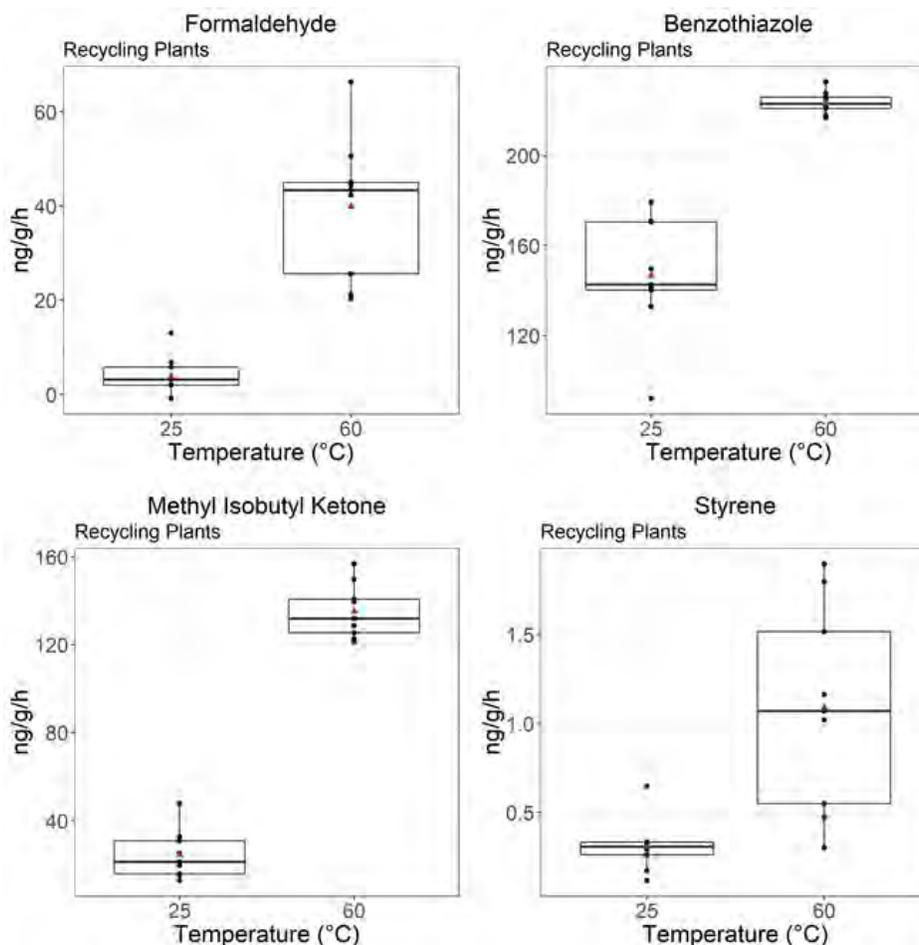
**Figure 4-27. Comparison of VOC 25 °C and 60 °C emission factor results (ng/g/h) for formaldehyde, benzothiazole, methyl isobutyl ketone, and styrene from tire crime rubber collected from recycling plants. [VOC = Volatile organic compound]**
