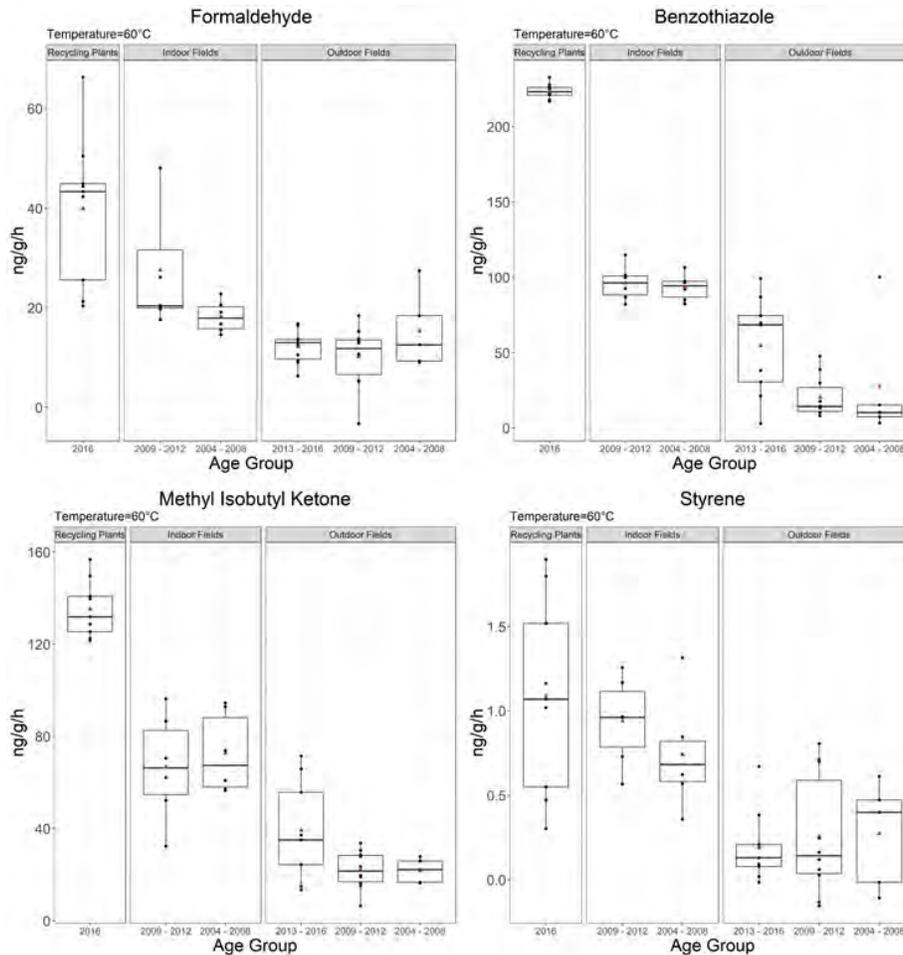
**Figure 4-53. Comparison of VOC 60 °C emission factor results (ng/g/h) between tire crumb rubber from recycling plants and tire crumb rubber infill composite samples from synthetic turf fields by age group for formaldehyde, benzothiazole, methyl isobutyl ketone, and styrene. [VOC = Volatile organic compound]**
