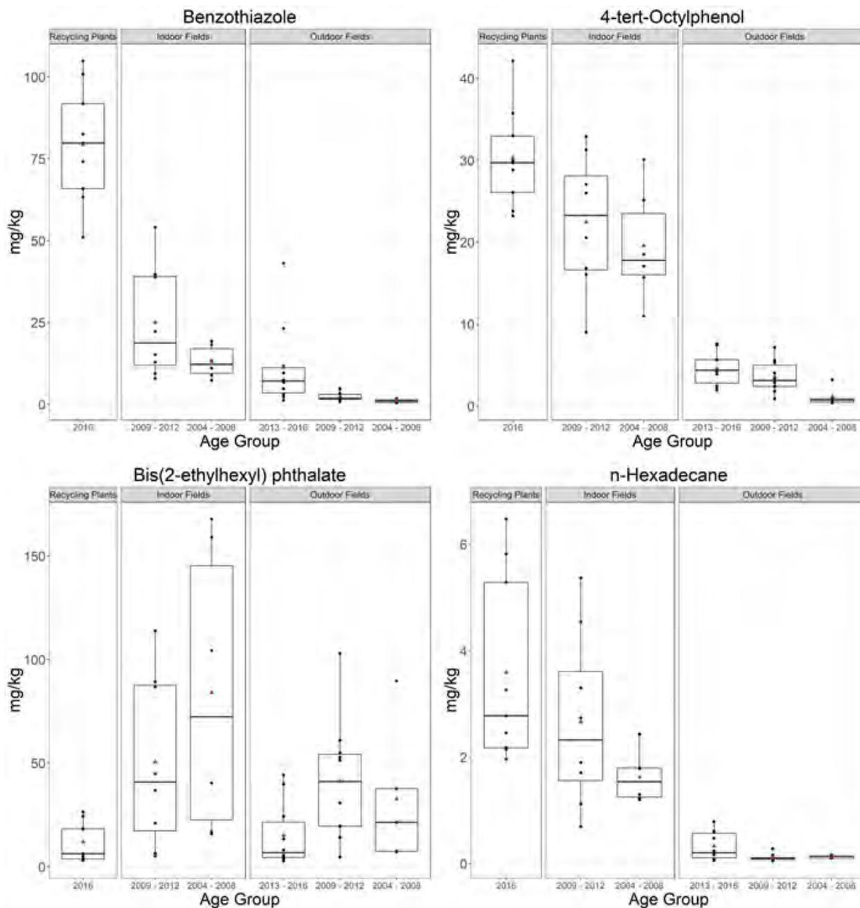
**Figure 4-51. Comparison of GC/MS/MS extract SVOC analysis results (mg/kg) between tire crumb rubber from recycling plants and tire crumb rubber infill composite samples from synthetic turf fields by age group for benzothiazole, 4-tert-octylphenol, bis(2-ethylhexyl) phthalate, and n-hexadecane. [GC/MS/MS = Gas chromatography/tandem mass spectrometry; SVOC = Semivolatile organic compound]**
