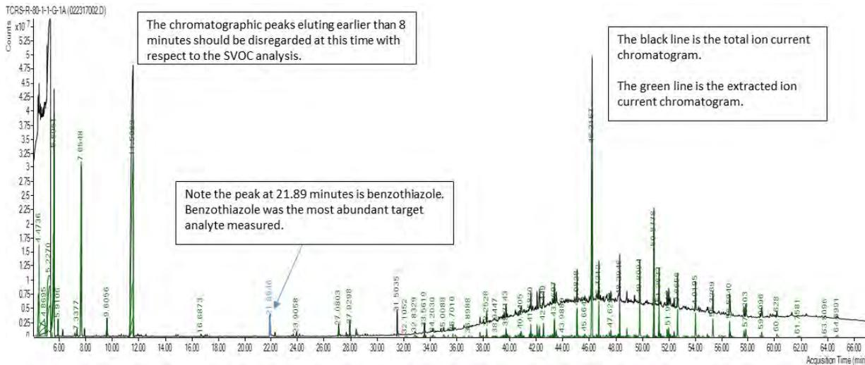
**Figure 4-63. Example GC/MS SVOC solvent extraction sample analysis showing total ion current and extracted ion current chromatograms for a recycling plant sample. [GC/MS = Gas chromatography/mass spectrometry; SVOC = Semivolatile organic compound]**
