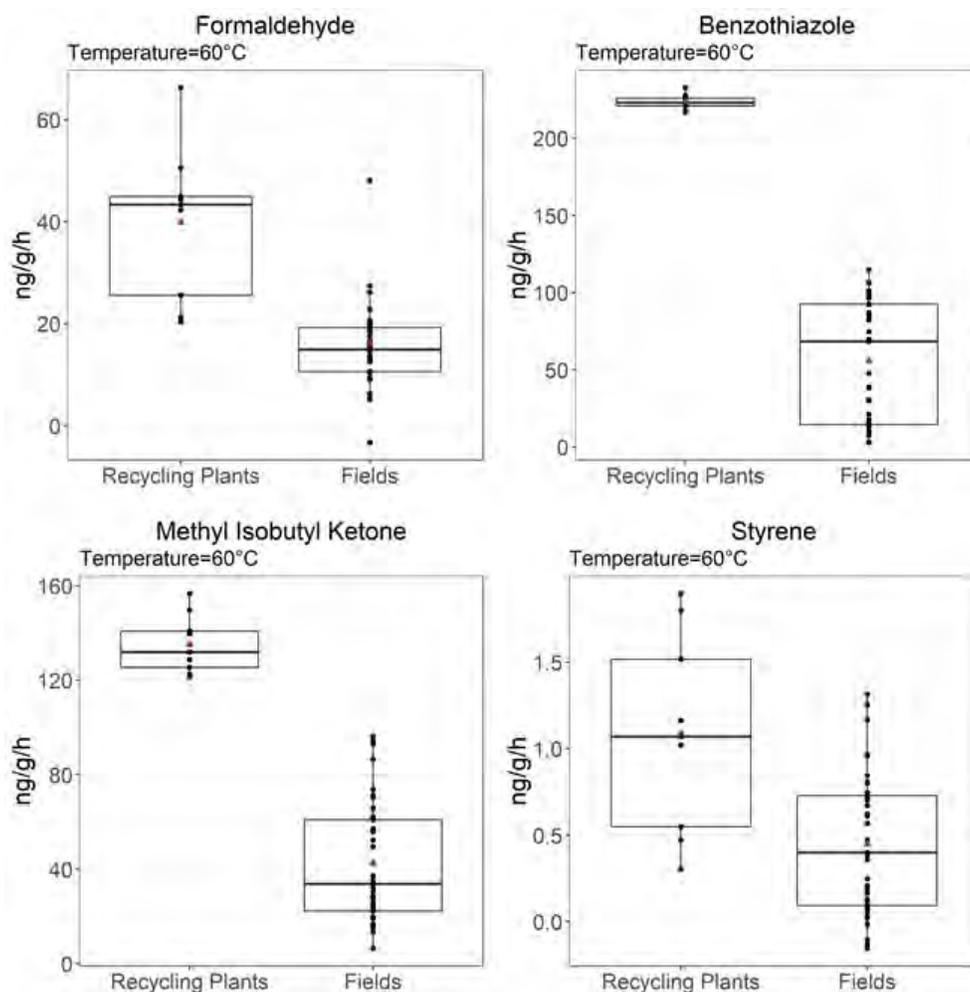
**Figure 4-25. Comparison of VOC 60 °C emission factor results (ng/g/h) between tire crumb rubber collected from tire recycling plants and tire crumb rubber infill composite samples from synthetic turf fields for formaldehyde, benzothiazole, methyl isobutyl ketone, and styrene. [VOC = Volatile organic compound]**
