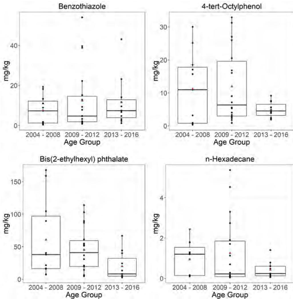
**Figure 4-45. Comparison of GC/MS/MS extract SVOC analysis results (mg/kg) between tire crumb rubber infill composite samples from synthetic turf fields in three installation age groups for benzothiazole, 4-tert-octylphenol, bis(2-ethylhexyl) phthalate, and n-hexadecane. [GC/MS/MS = Gas chromatography/tandem mass spectrometry; SVOC = Semivolatile organic compound]**
