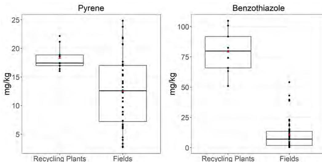
**Figure 2-8. Example comparison of GC/MS/MS extract SVOC analysis results (mg/kg) between tire rubber collected from tire recycling plants and tire crumb rubber infill composite samples from synthetic turf fields for pyrene and benzothiazole.**
