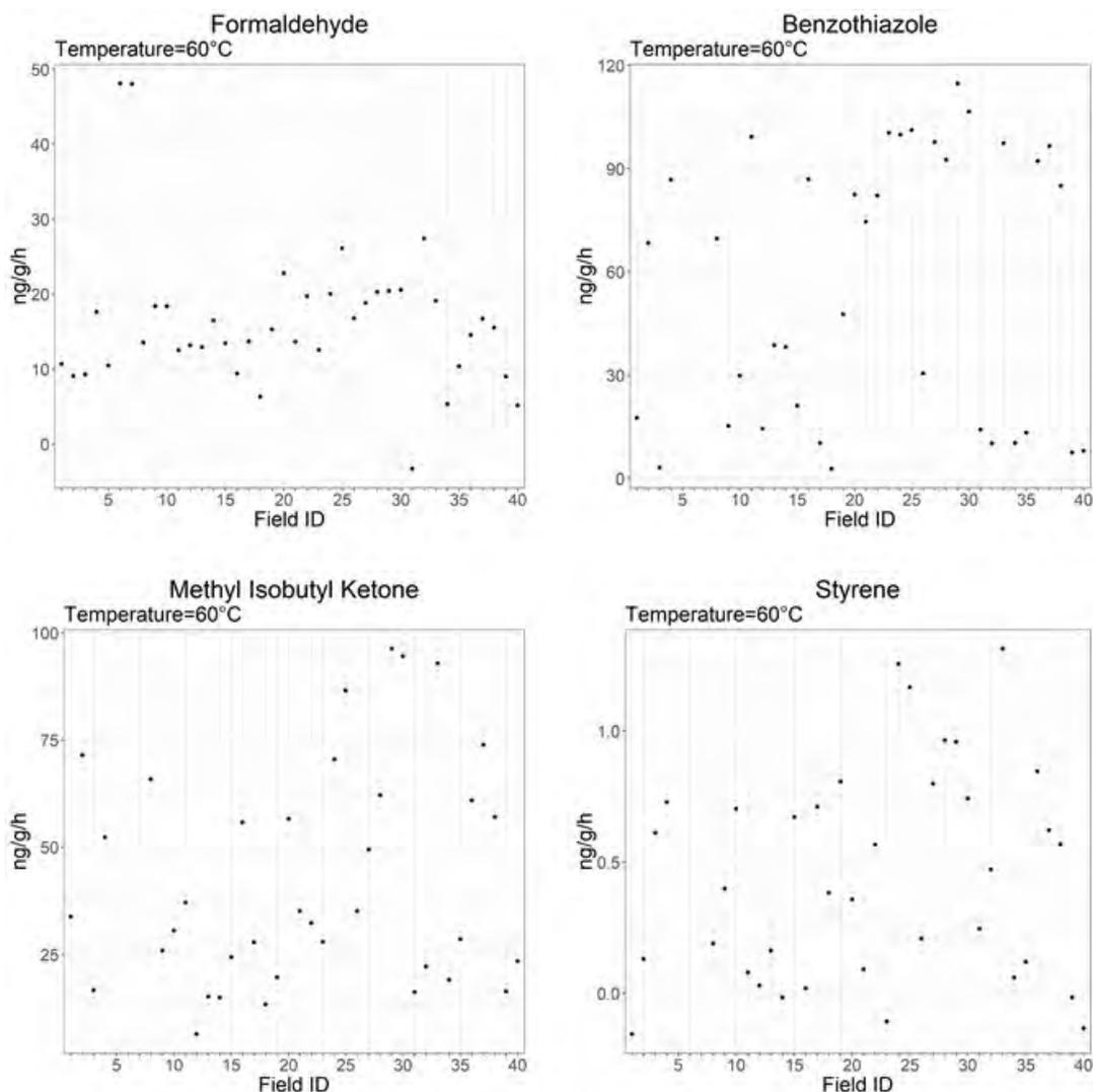
**Figure 4-17. VOC 60 °C emission factor results (ng/g/h) for formaldehyde, benzothiazole, methyl isobutyl ketone, and styrene from tire crumb rubber infill composite samples collected from each synthetic turf field. [VOC = Volatile organic compound]**
