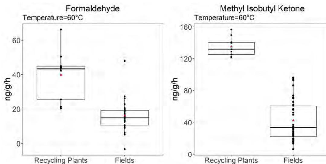
**Figure 2-12. Comparison of volatile organic compound 60 °C emission factor results (ng/g/h) between tire rubber collected from tire recycling plants and tire crumb rubber infill composite samples from synthetic turf fields for formaldehyde and methyl isobutyl ketone.**
