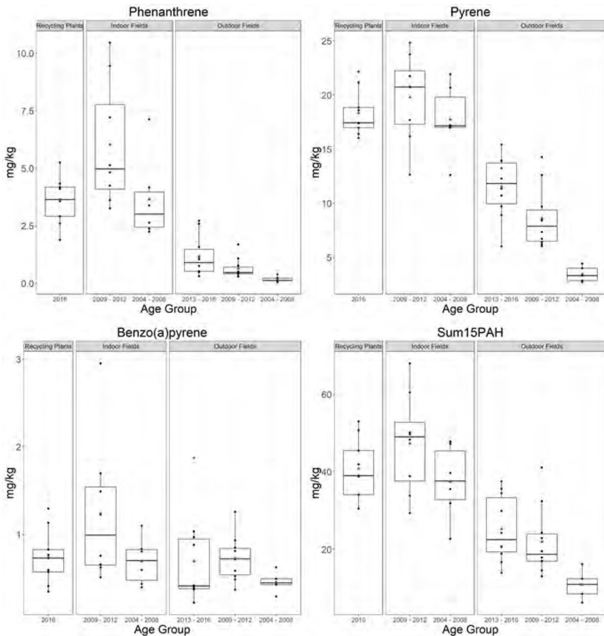
**Figure 4-50. Comparison of GC/MS/MS extract SVOC analysis results (mg/kg) between tire crumb rubber from recycling plants and tire crumb rubber infill composite samples from synthetic turf fields by age group for phenanthrene, pyrene, benzo(a)pyrene, and the sum of 15 PAHs. [GC/MS/MS = Gas chromatography/tandem mass spectrometry; SVOC = Semivolatile organic compound]**
