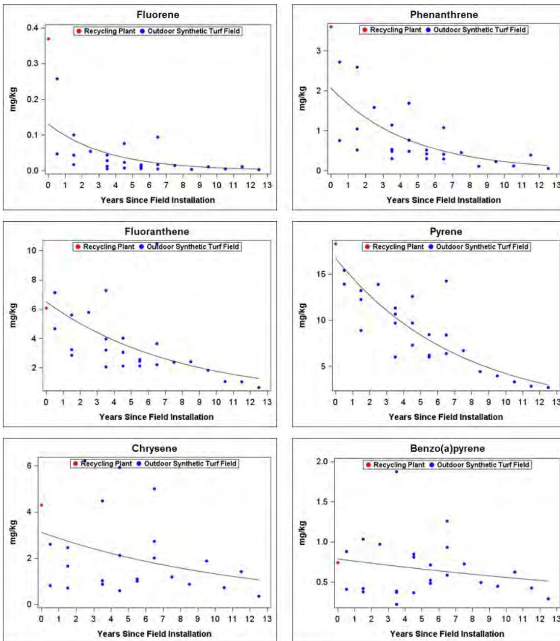
**Figure 4-55. Concentrations of select extractable PAHs in outdoor field composite tire crumb rubber infill samples versus years since field installation. The average concentration for the recycling plant tire crumb rubber is also shown on each graph as a zero point for time. The modeled relationships between the concentrations and years are shown as curves. [PAH = Polycyclic aromatic hydrocarbons]**
