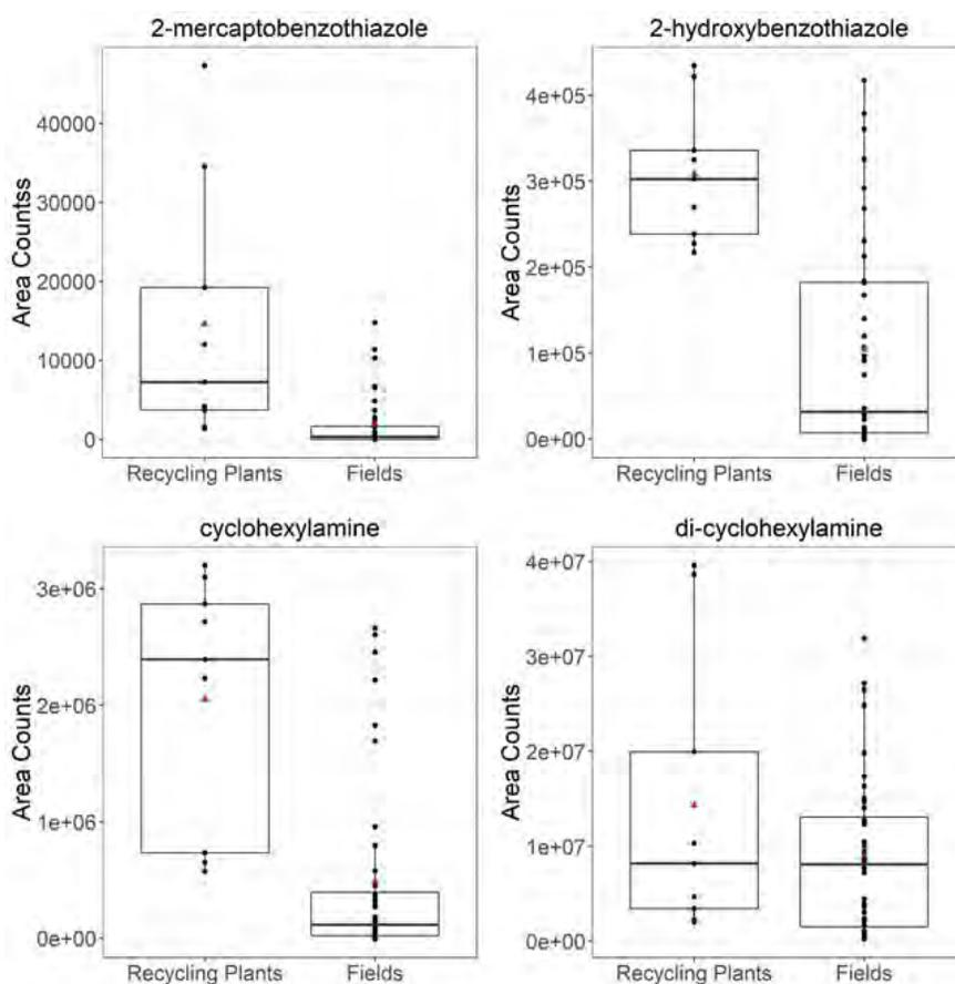
**Figure 4-24. Comparison of LC/TOFMS positive ionization extract SVOC non-quantitative analysis results (chromatographic area counts) between tire crumb rubber collected from tire recycling plants and tire crumb rubber infill composite samples from synthetic turf fields for 2-mercaptobenzothiazole, 2-hydroxybenzothiazole, cyclohexylamine, and di-cyclohexylamine. [SVOC = Semivolatile organic compound; LC/TOFMS = Liquid chromatography/time-of-flight mass spectrometry]**
