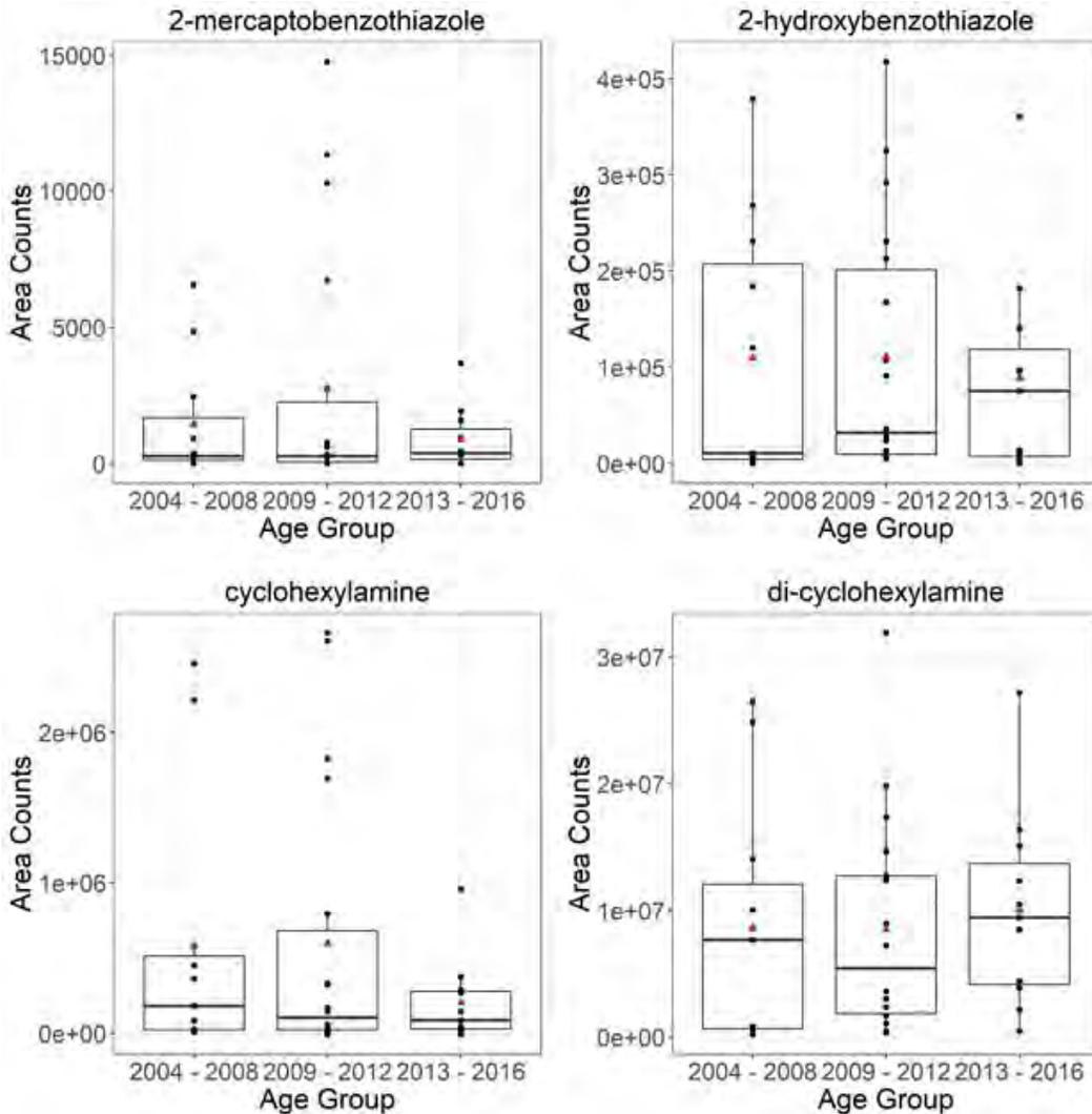
**Figure 4-46. Comparison of LC/TOFMS extract SVOC non-quantitative positive ionization analysis results between tire crumb rubber infill composite samples from synthetic turf fields in three installation age groups for 2-mercaptobenzothiazole, 2-hydroxybenzothiazole, cyclohexylamine, and di-cyclohexylamine. [LC/TOFMS = Liquid chromatography/time-of-flight mass spectrometry; SVOC = Semivolatile organic compound]**
