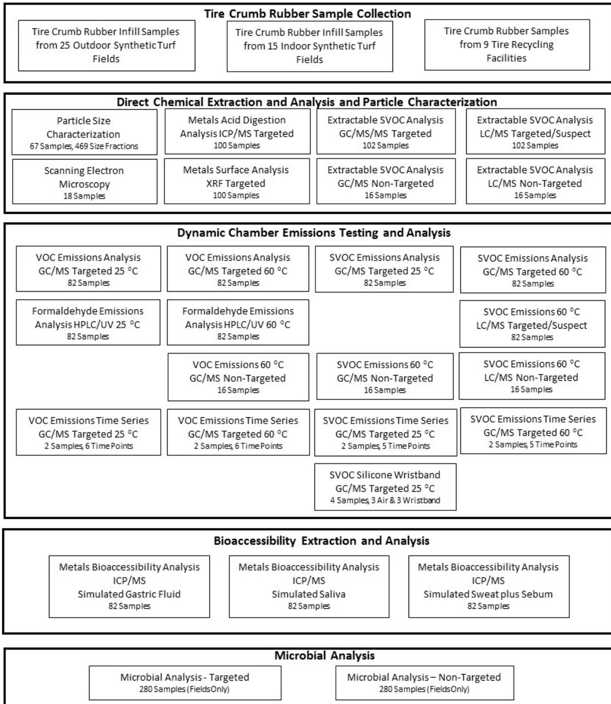
**Figure 3-1. Tire crumb rubber characterization research schematic overview.**
