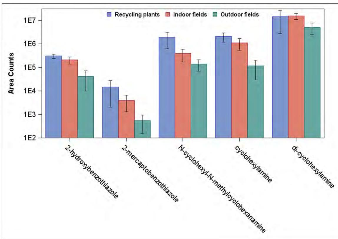
**Figure 2-7.** Average relative chromatographic peak area count results for select semivolatile organic compounds in solvent extraction samples from tire crumb rubber collected at tire recycling plants (n=9), indoor synthetic turf fields (n=15), and outdoor synthetic turf fields (n=25). These results are not quantitative, but compound identities were confirmed.
