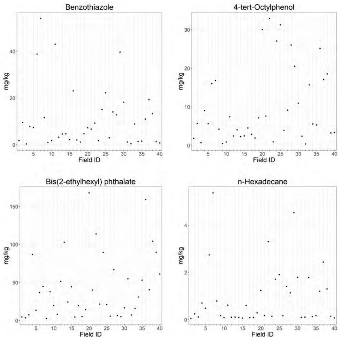
**Figure 4-16. GC/MS/MS extract analysis results (mg/kg) for benzothiazole, 4-tert-octylphenol, bis(2-ethylhexyl) phthalate, and n-hexadecane from tire crumb rubber infill composite samples collected from each synthetic turf field. [GC/MS/MS = Gas chromatography/tandem mass spectrometry]**
