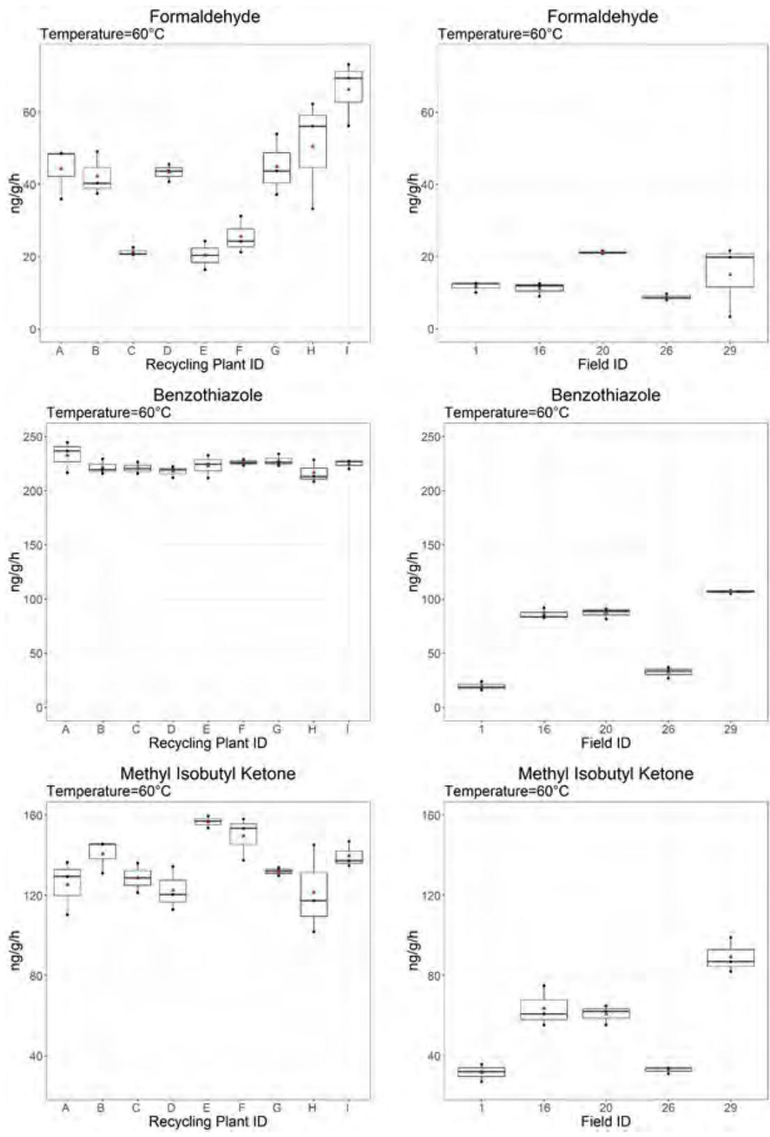
**Figure 4-35. Within-tire recycling plant variability (left side) and within-synthetic turf field variability (right side) variability for VOC emission factor 60 °C analysis results (ng/g/h) in tire crumb rubber for formaldehyde, benzothiazole, and methyl isobutyl ketone. [VOC = Volatile organic compound]**
