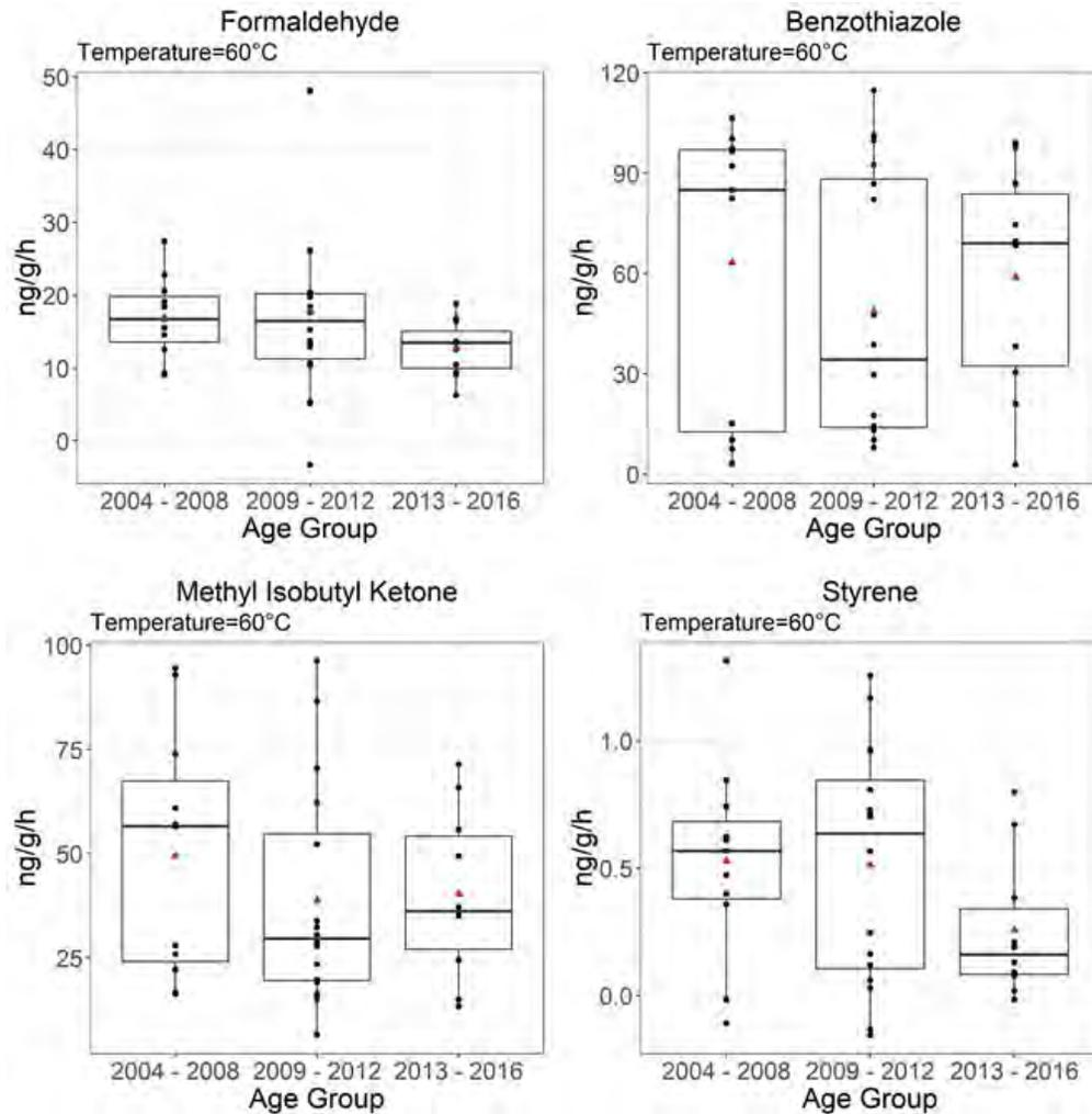
**Figure 4-47. Comparison of VOC 60 °C emission factor results (ng/g/h) between tire crumb rubber infill composite samples from synthetic turf fields in three installation age groups for formaldehyde, benzothiazole, methyl isobutyl ketone, and styrene. [VOC = Volatile organic compound]**
