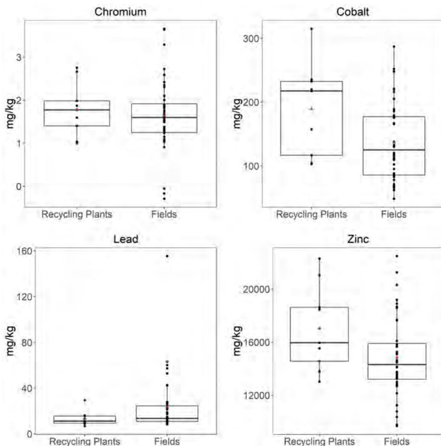
**Figure 4-21. Comparison of ICP/MS metal analysis results (mg/kg) between tire crumb rubber collected from tire recycling plants and tire crumb rubber infill composite samples from synthetic turf fields for chromium, cobalt, lead, and zinc.** [ICP/MS = Inductively coupled plasma/mass spectrometry]
