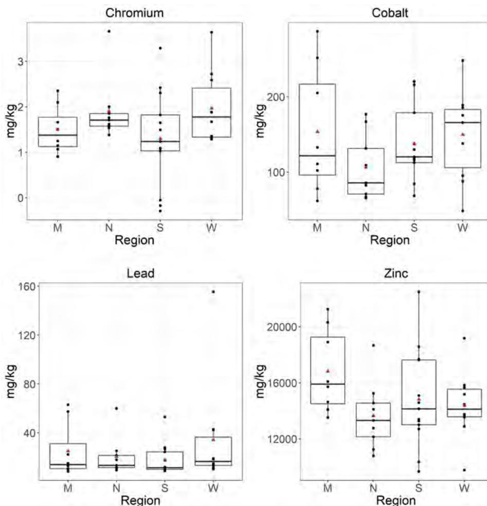
**Figure 4-57. Comparison of ICP/MS metal analysis results (mg/kg) between tire crumb rubber infill composite samples from synthetic turf fields in four U.S. census regions for chromium, cobalt, lead, and zinc.** [ICP/MS = Inductively coupled plasma/mass spectrometry; M = Midwest; N = Northeast; S = South; W = West]
