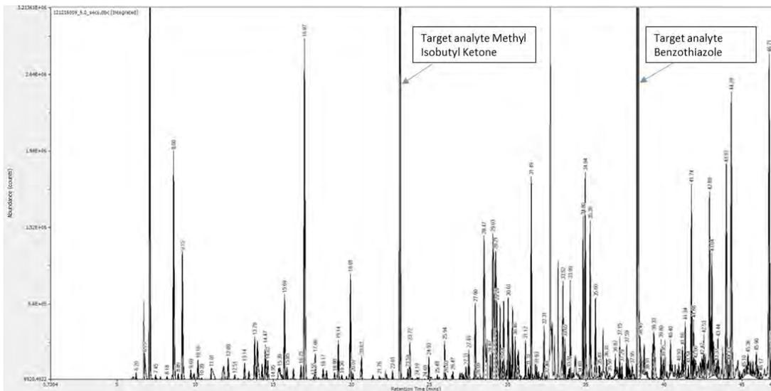
**Figure 4-64. Example GC/TOFMS VOC 60 °C chamber emission sample analysis total ion current chromatogram for a synthetic turf field. [GC/TOFMS = Gas chromatography/time-of-flight mass spectrometry; VOC = Volatile organic compound]**
