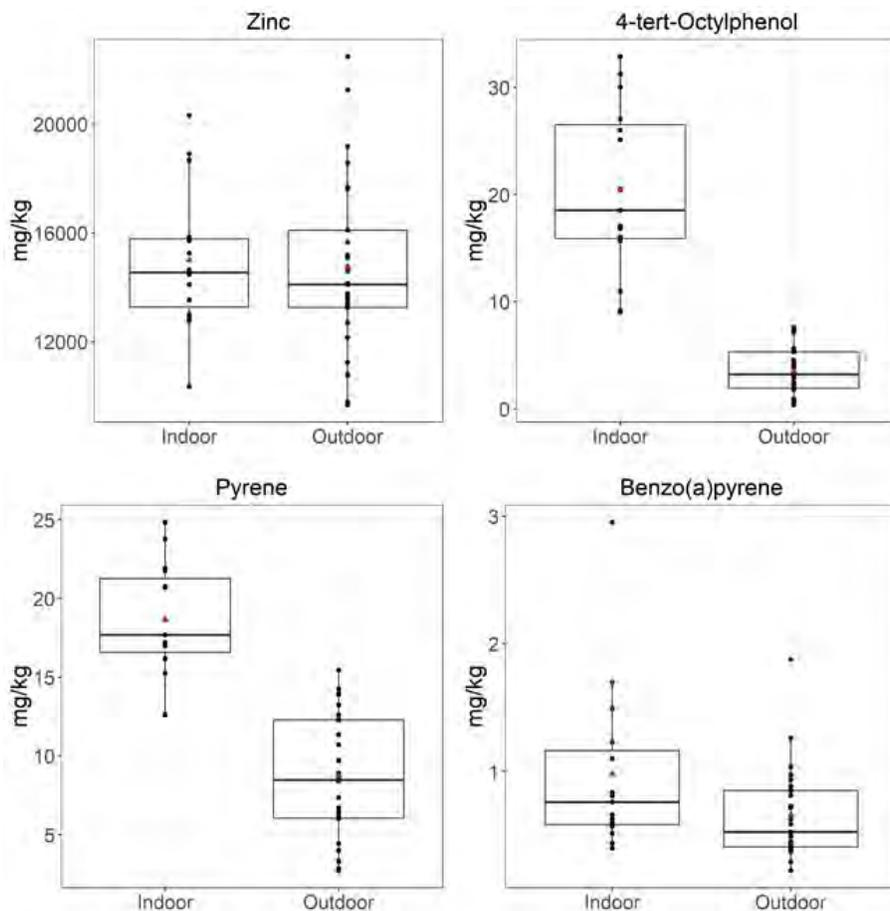
**Figure 2-9. Comparison of analysis results (mg/kg) between tire crumb rubber infill composite samples from indoor and outdoor synthetic turf fields for zinc, 4-tert-octylphenol, pyrene and benzo[a]pyrene.**
