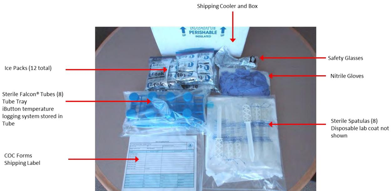
**Figure 3-9. Sample collection kit for microbial sample collection at synthetic turf fields.**
