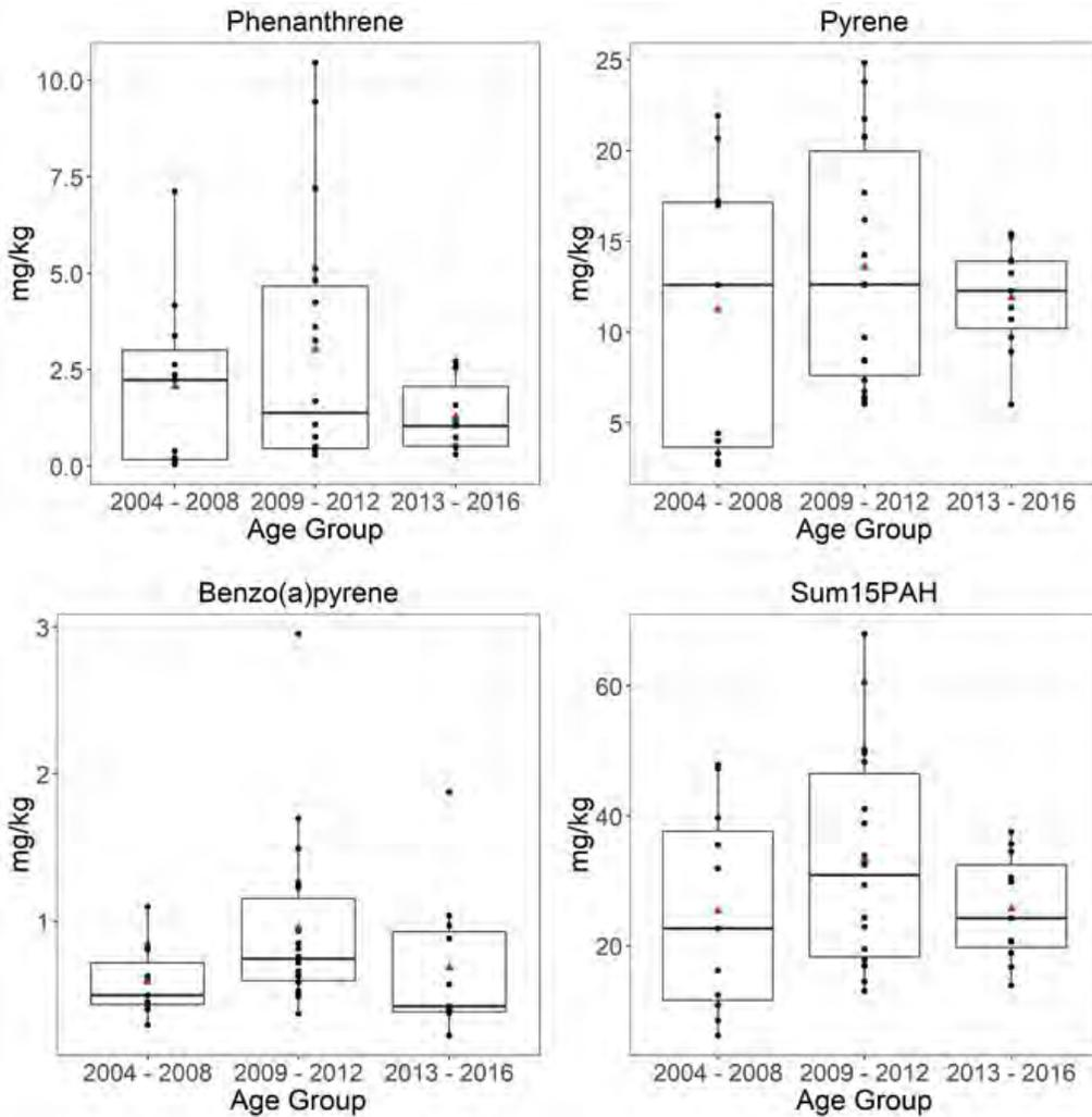
**Figure 4-44. Comparison of GC/MS/MS extract SVOC analysis results (mg/kg) between tire crumb rubber infill composite samples from synthetic turf fields in three installation age groups for phenanthrene, pyrene, benzo[a]pyrene, and the sum of 15 PAHs.**
