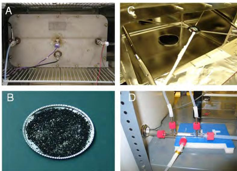
**Figure 3-12. Small emission chamber set-up, including A) sealed 53-L chamber in incubator cabinet; B) 15 g tire crumb rubber infill sample prepared for testing; C) chamber interior with sample in place and mixing fan pulled out; D) external manifold for air sample collection.**
