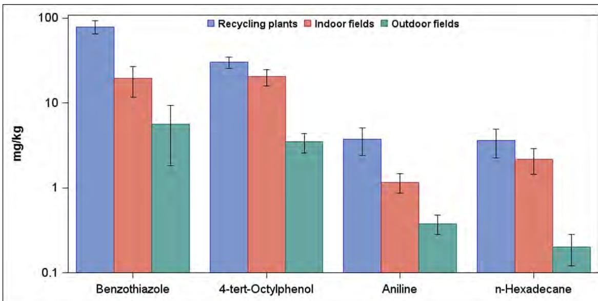
**Figure 2-6.** Average measurement results for select semivolatile organic compounds in solvent extraction samples from tire crumb rubber collected at tire recycling plants (n=9), indoor synthetic turf fields (n=15), and outdoor synthetic turf fields (n=25).
