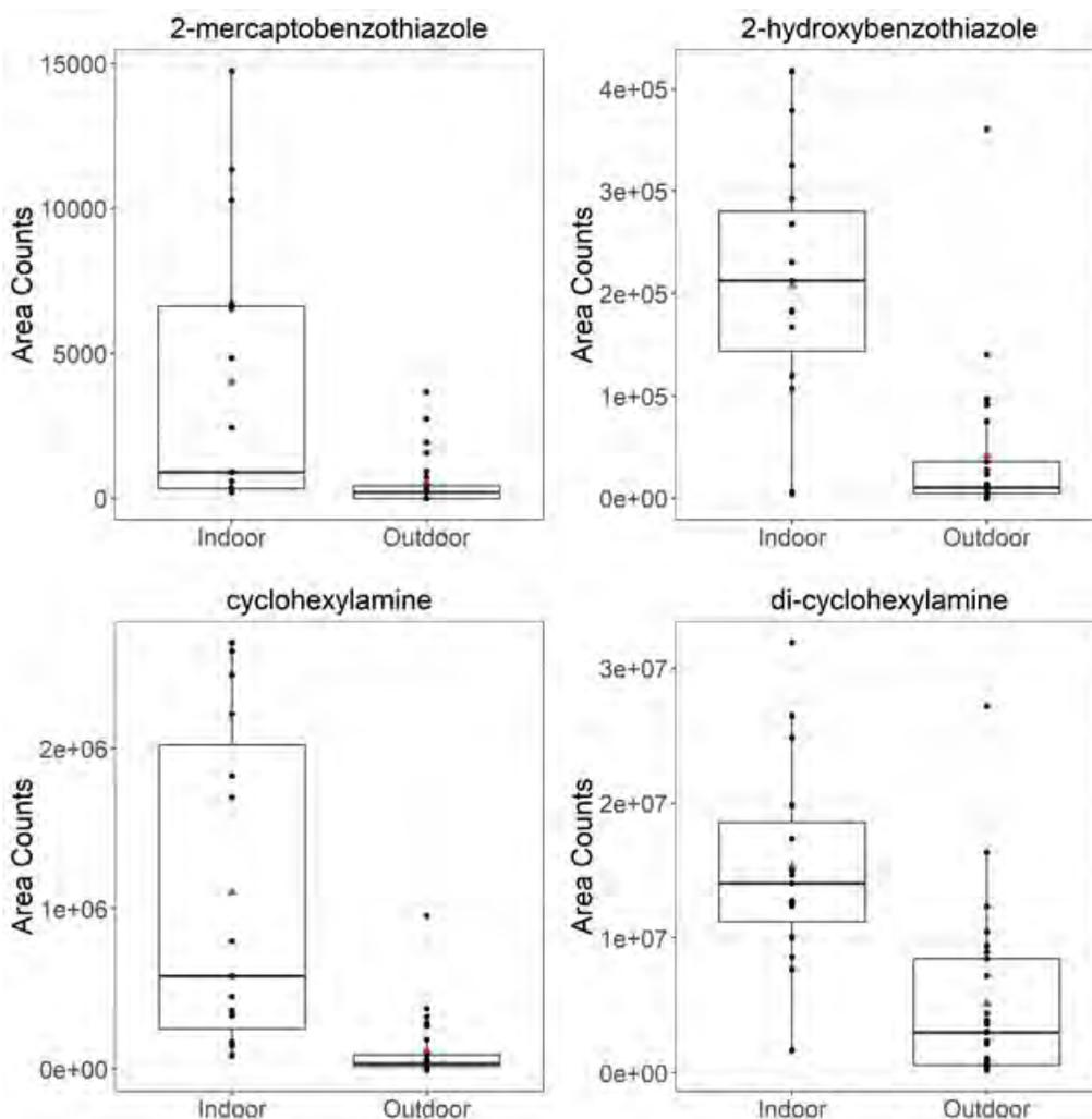
**Figure 4-40. Comparison of LC/TOFMS extract SVOC non-quantitative positive ionization analysis results between tire crumb rubber infill composite samples from indoor and outdoor synthetic turf fields for 2-mercaptobenzothiazole, 2-hydroxybenzothiazole, cyclohexylamine, di-cyclohexylamine.** [LC/TOFMS = Liquid chromatography/time-of-flight mass spectrometry; SVOC = Semivolatile organic compound]
