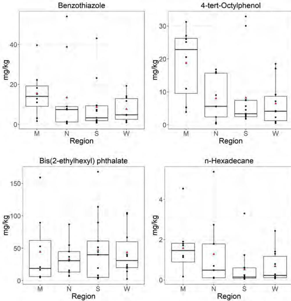
**Figure 4-59. Comparison of GC/MS/MS extract SVOC analysis results (mg/kg) between tire crumb rubber infill composite samples from synthetic turf fields in four U.S. census regions for benzothiazole, 4-tert-octylphenol, bis(2-ethylhexyl) phthalate, and n-hexadecane.** [GC/MS/MS = Gas chromatography/tandem mass spectrometry; SVOC = Semivolatile organic compound; M = Midwest; N = Northeast; S = South; W = West]
