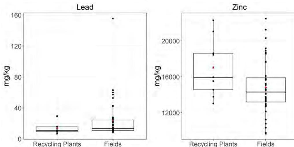
**Figure 2-4. ICP/MS metal analysis results (mg/kg) for tire crumb rubber collected from tire recycling plants and tire crumb rubber infill composite samples from synthetic turf fields for lead and zinc.**
