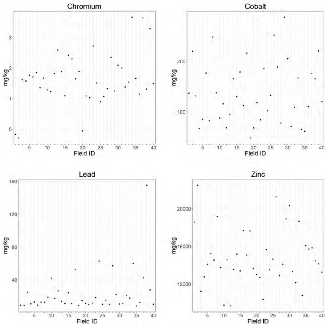
**Figure 4-14. ICP/MS metal analysis results (mg/kg) for chromium, cobalt, lead, and zinc from tire crumb rubber infill composite samples collected from each synthetic turf field.**
