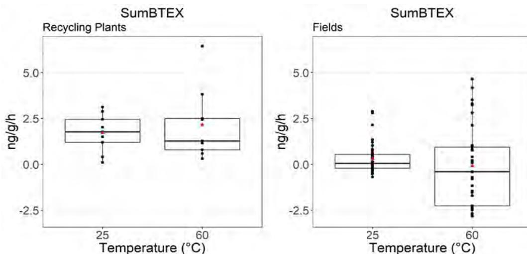
**Figure 4-29. Comparison of VOC 25 °C and 60 °C emission factor results (ng/g/h) for SumBTEX from tire crumb rubber collected from recycling plants and tire crumb rubber infill collected from synthetic turf fields.** [VOC = Volatile organic compound; SumBTEX = Sum of benzene, toluene, ethylbenzene, m/p-xylene, and o-xylene results]
