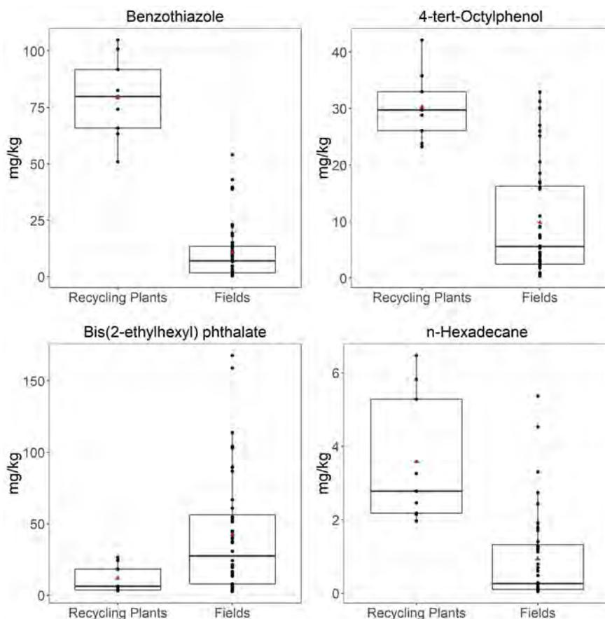
**Figure 4-23. Comparison of GC/MS/MS extract SVOC analysis results (mg/kg) between tire crumb rubber collected from tire recycling plants and tire crumb rubber infill composite samples from synthetic turf fields for benzothiazole, 4-tert-octylphenol, bis(2-ethylhexyl) phthalate, and n-hexadecane.** [SVOC = Semivolatile organic compound; GC/MS/MS = Gas chromatography/tandem mass spectrometry]
