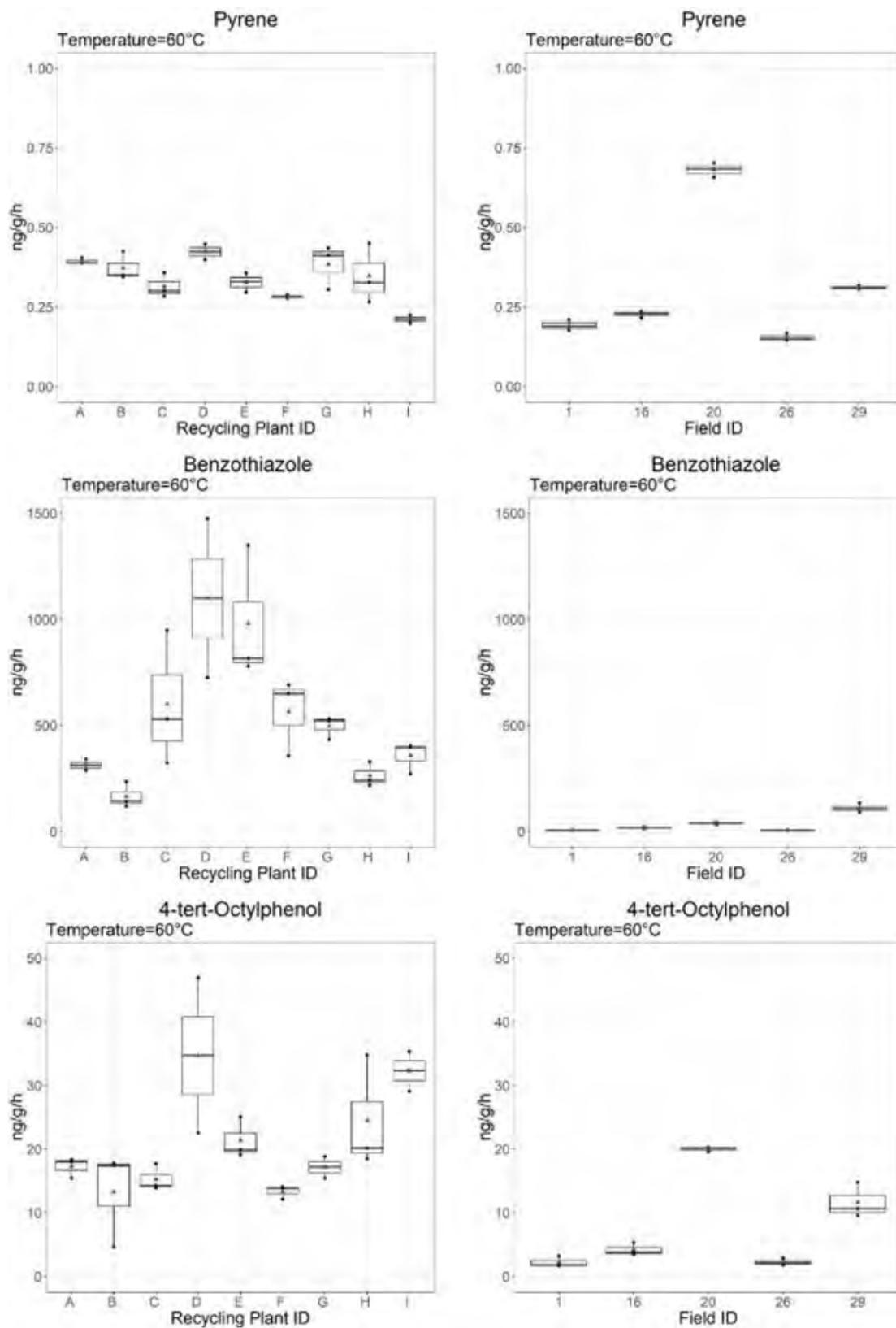
**Figure 4-36. Within-tire recycling plant variability (left side) and within-synthetic turf field variability (right side) variability for SVOC emission factor 60 °C analysis results (ng/g/h) in tire crumb rubber for pyrene, benzothiazole, 4-tert-octylphenol. [SVOC = Semivolatle organic compound]**
