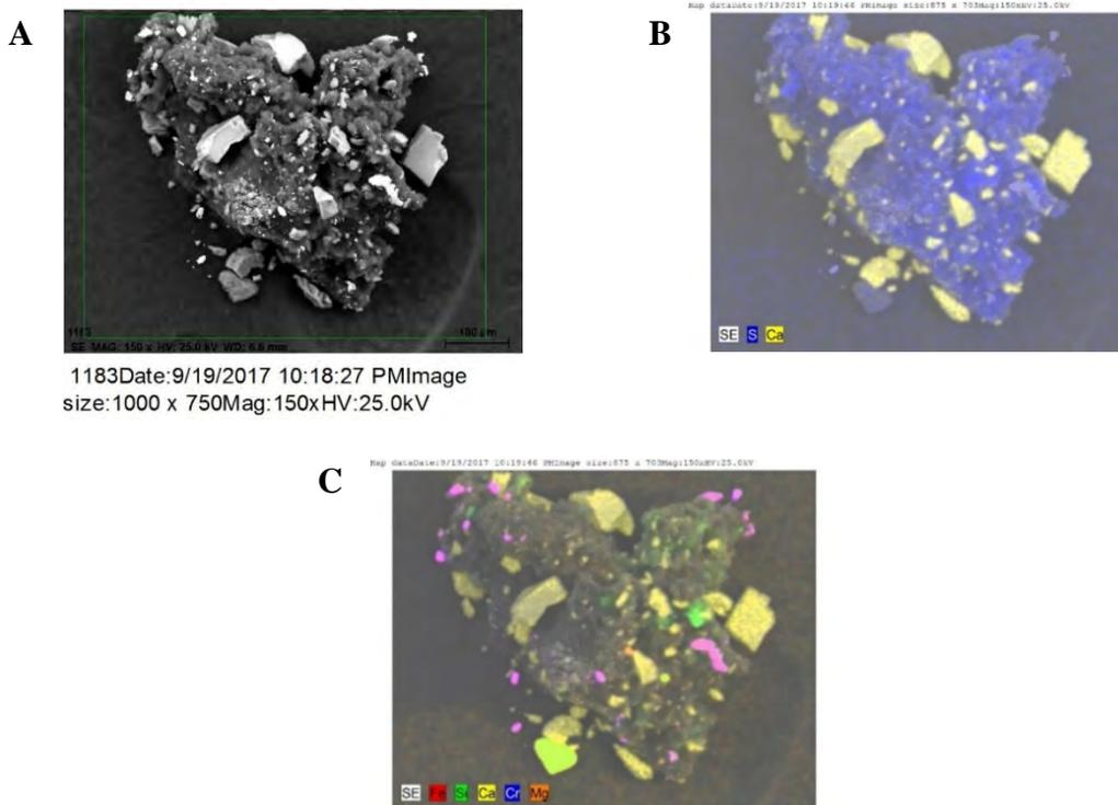
**Figure 4-12. Three EPMA element mapping images. A) Original electron micrograph; B) Sulfur map indicating primary rubber particle; and C) multielement map showing inclusions probably steel (Fe+Cr) and possibly soil (Si, Ca).** [EPMA = Electron probe microanalysis; Ca = Calcium; Cr = Chromium; Fe = Iron; Mg = Magnesium; S = Sulfur; Si = Silicon]
