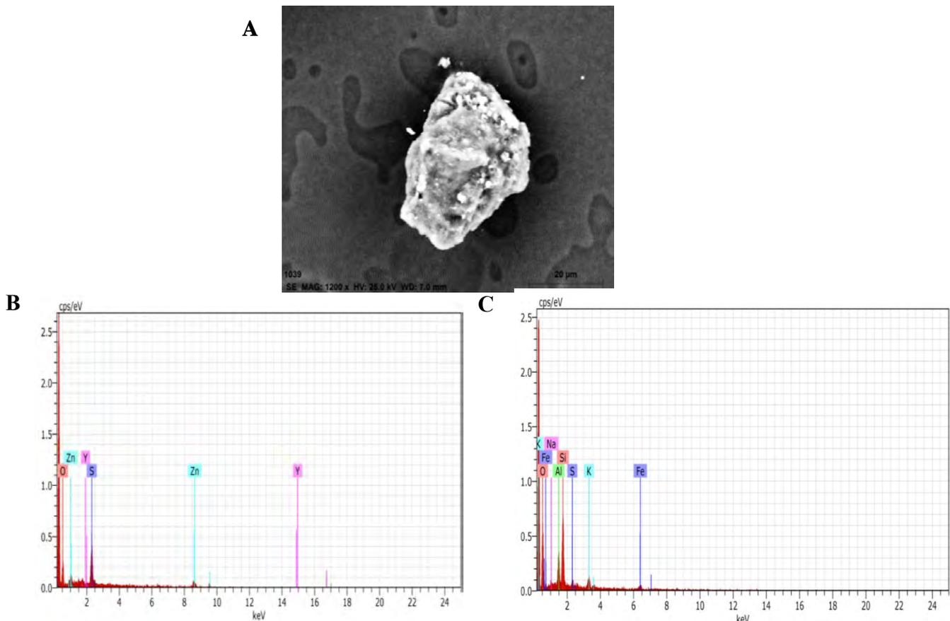
**Figure 4-11. A) Electron micrograph of small particle cluster from a field sample; B) EPMA spectrum of the center of the large center particle; C) Spectrum of smaller particle above the central particle. [EPMA = Electron probe microanalysis; Al = Aluminum; Fe = Iron; K = Potassium; Na = Sodium; O = Oxygen; S = Sulfur; Si = Silicon; Y = Yttrium; Zn = Zinc]**
