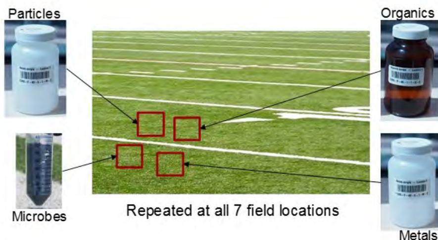
**Figure 3-7. Schematic representation of the four samples that were collected at each of the seven locations on each field. Samples for chemical and particle characterization were collected into 250-mL pre-cleaned amber glass or high-density polyethylene (HDPE) jars. Microbial samples were collected into sterile 50-mL tubes.**
