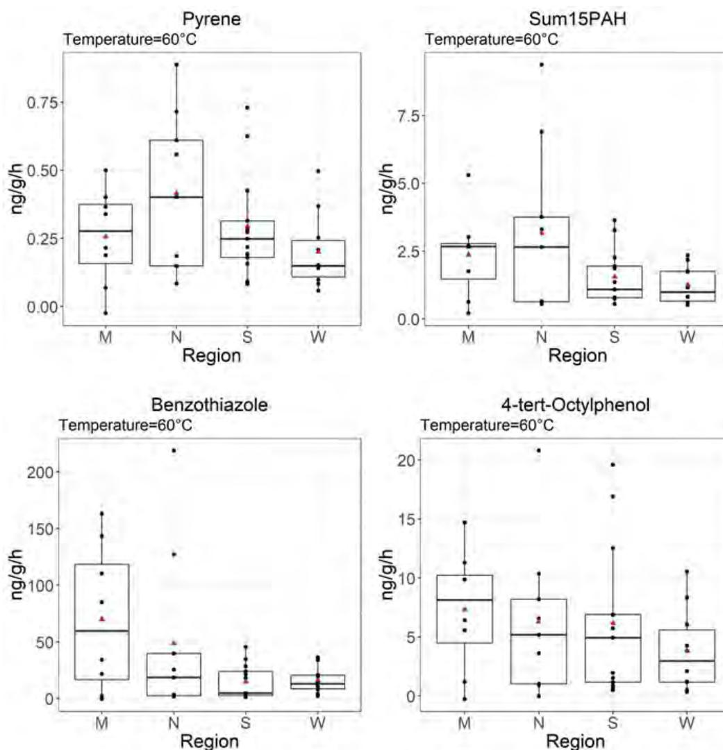
**Figure 4-62. Comparison of SVOC 60 °C emission factor results (ng/g/h) between tire crumb rubber infill composite samples from synthetic turf fields in four U.S. census regions for pyrene, the sum of 15 PAHs, benzothiazole, and 4-tert-octylphenol.**
