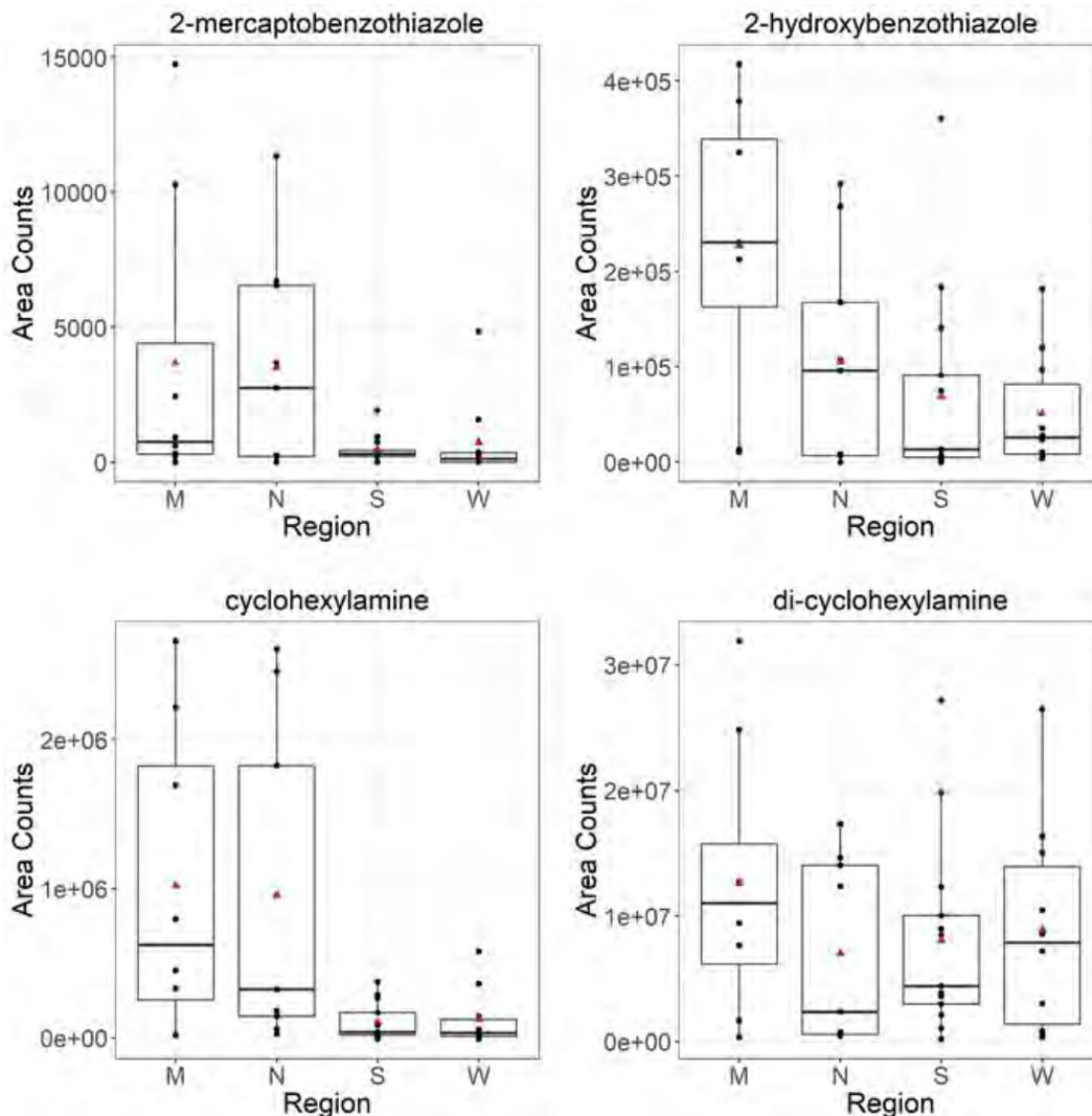
**Figure 4-60. Comparison of LC/TOFMS extract SVOC non-quantitative positive ionization analysis results between tire crumb rubber infill composite samples from synthetic turf fields in four U.S. census regions for 2-mercaptobenzothiazole, 2-hydroxybenzothiazole, cyclohexylamine, di-cyclohexylamine.** [LC/TOFMS = Liquid chromatography/time-of-flight mass spectrometry; SVOC = Semivolatile organic compound; M = Midwest; N = Northeast; S = South; W = West]
