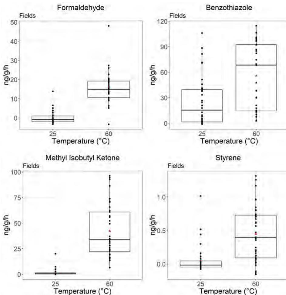
**Figure 4-28. Comparison of VOC 25 °C and 60 °C emission factor results (ng/g/h) for formaldehyde, benzothiazole, methyl isobutyl ketone, and styrene from tire crumb rubber infill collected from synthetic turf fields. [VOC = Volatile organic compound]**
