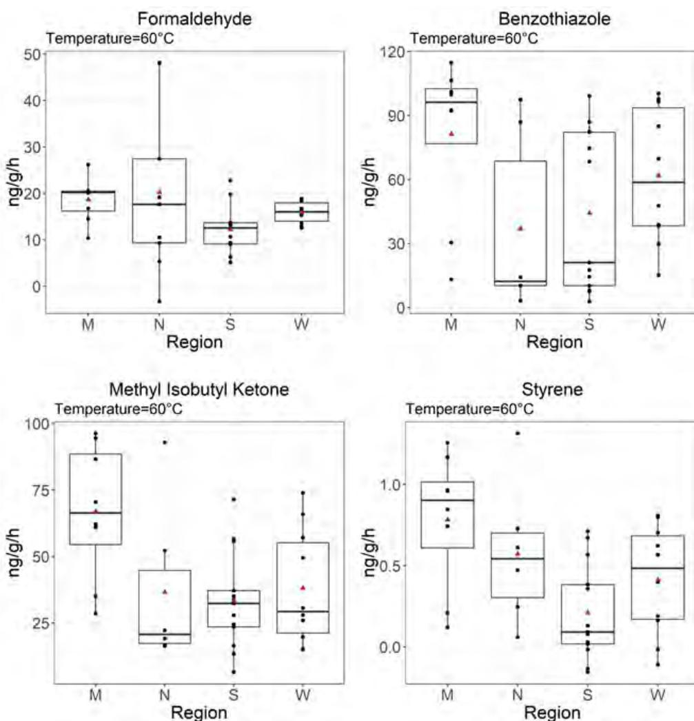
**Figure 4-61. Comparison of VOC 60 °C emission factor results (ng/g/h) between tire crumb rubber infill composite samples from synthetic turf fields in four U.S. census regions for formaldehyde, benzothiazole, methyl isobutyl ketone, and styrene. [VOC = Volatile organic compound; M = Midwest; N = Northeast; S = South; W = West]**
