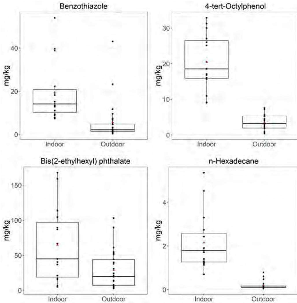
**Figure 4-39. Comparison of GC/MS/MS extract SVOC analysis results (mg/kg) between tire crumb rubber infill composite samples from indoor and outdoor synthetic turf fields for benzothiazole, 4-tert-octylphenol, bis(2-ethylhexyl) phthalate, and n-hexadecane. [GC/MS/MS = Gas chromatography/tandem mass spectrometry; SVOC = Semivolatile organic compound]**
