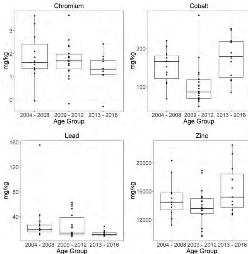
**Figure 4-43. Comparison of ICP/MS metal analysis results (mg/kg) between tire crumb rubber infill composite samples from synthetic turf fields in three installation age groups for chromium, cobalt, lead, and zinc.**
