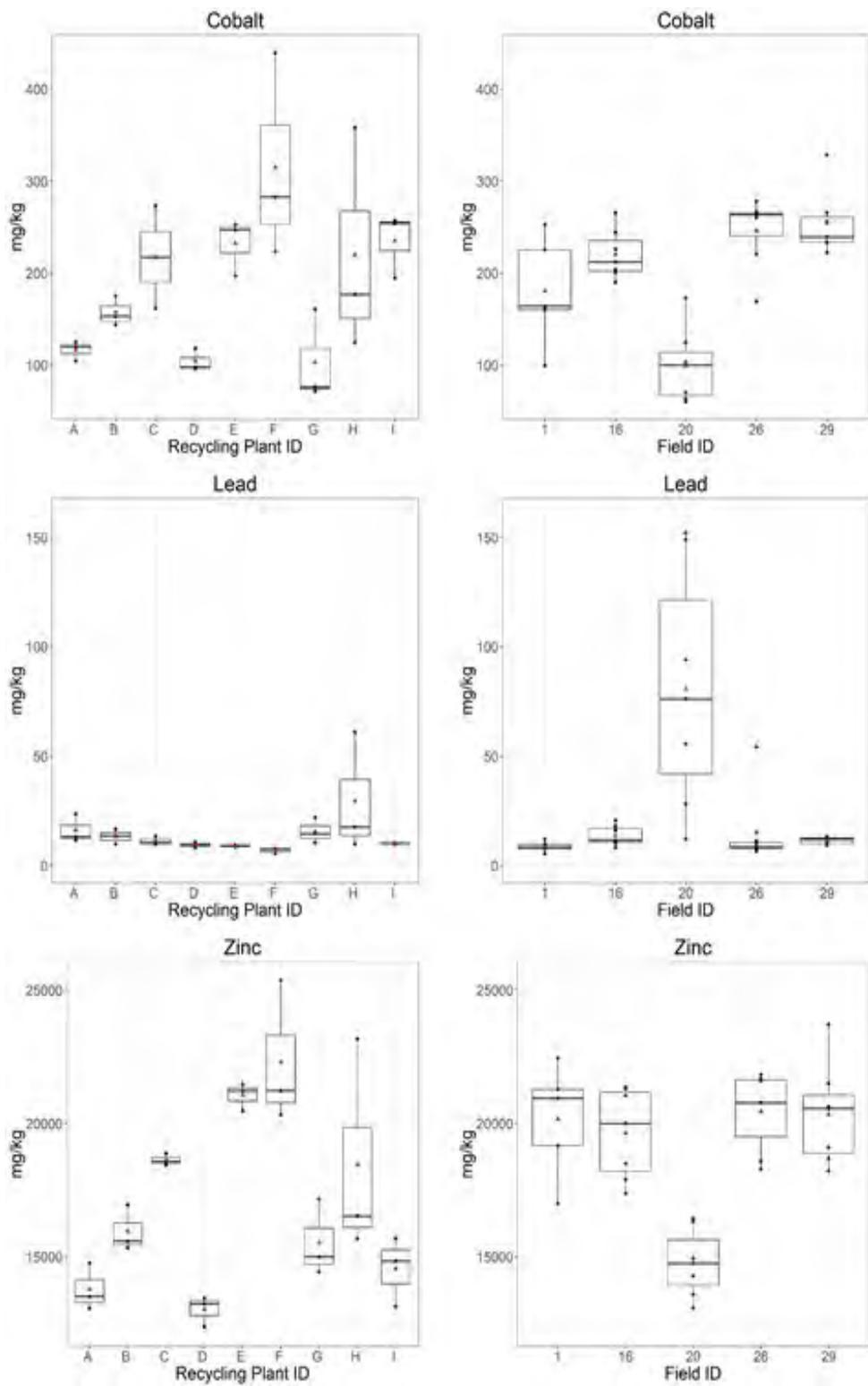
**Figure 4-32. Within-tire recycling plant variability (left side) and within-synthetic turf field variability (right side) for ICP/MS metal analysis results (mg/kg) in tire crumb rubber for cobalt, lead, and zinc. [ICP/MS = Inductively coupled plasma/mass spectrometry]**
