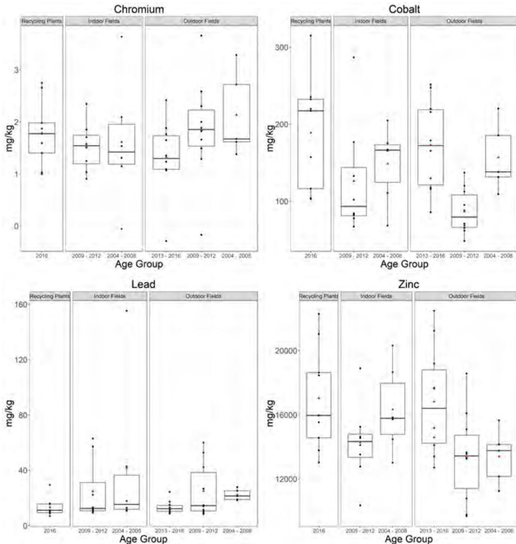
**Figure 4-49. Comparison of ICP/MS metal analysis results (mg/kg) between tire crumb rubber from recycling plants and tire crumb rubber infill composite samples from synthetic turf fields by age group for chromium, cobalt, lead, and zinc. [ICP/MS = Inductively coupled plasma/mass spectrometry]**
